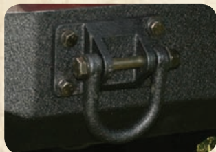
D-rings attach securely to the frame of the vehicle for a rock solid recovery mounting point.
